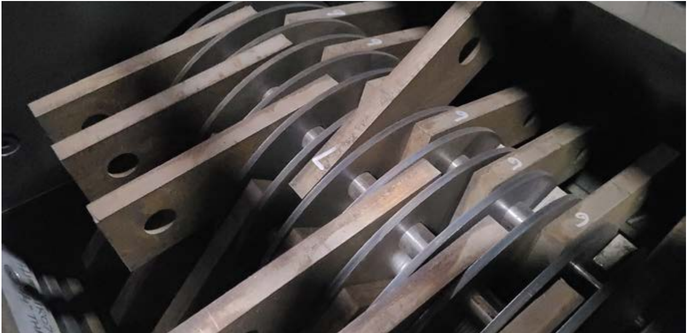
WA Series rotor assembly featuring optional tungsten carbide coated hammers for highly abrasive applications.
