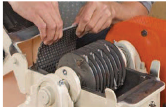
Mill top hinges open for easy screen change and mill maintenance
