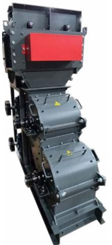
The Patent Pending DataKiller ProTM, a One Pass Data and Electronics Destroyer, features a unique dual shaft rip shredder integrated with a dual stage hammer mill. This unique design is ideal for super-fine electronic scrap grinding, under 2MM, at very high production rates and at previously unheard of volume reduction ratios. As a result, a sub-2mm grind is achieved in one pass through the DataKiller Pro.
