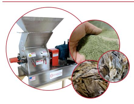
Schutte Hammermill Mini Mills are the perfect solution for the processing of dried seaweed and kelp. The Mini Mills offer the same operational capability of larger size reduction equipment with a much smaller footprint. The Mini Mills promise uniform output sizes for food, cosmetics and many othe applications. We offer options in carbon steel and stainless steel with various surface finishes.
