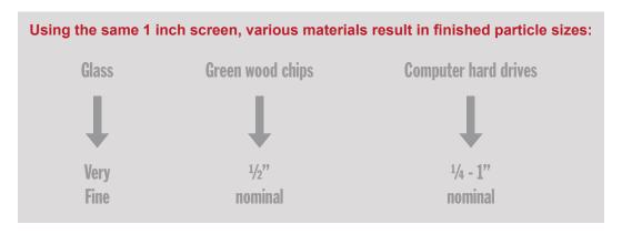
This variation is called particle size distribution, and it is based on the individual properties of the materials being processed.
