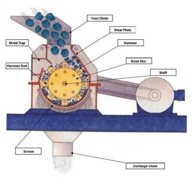
Hammer mills operate on the basic principle that most materials will crush, shatter or pulverize upon impact. This is accomplished by a simple four step process:
