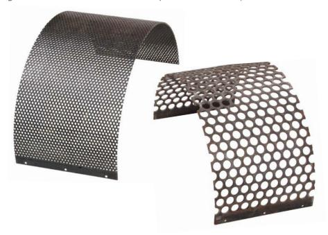
The appropriate screen size is determined by the desired finished particle size, and the properties of the material being processed. That is, characteristics such as friability and moisture content have an effect of the manner in which a material will break down. As a result, using the same screen to process materials of different properties will result in a range of different finished particle sizes.
