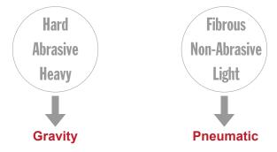
It's all about the fan. Air swept mills are used primarily when grinding light, relatively non-abrasive materials to a mid range to fine particle size because lighter particles require suction to overcome the rotor airflow. The fan pulls the material from the mill in-feed through the grinding chamber. In addition, it pulls the finished product through the suction pipe, into the fan itself, and then blows the material out of the discharge pipe either to storage or next stage of processing.
