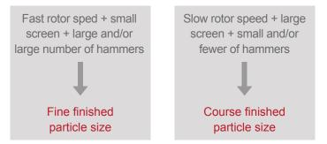
Each of these components can be changed either individually or in combination to produce the exact desired finished particle size.
