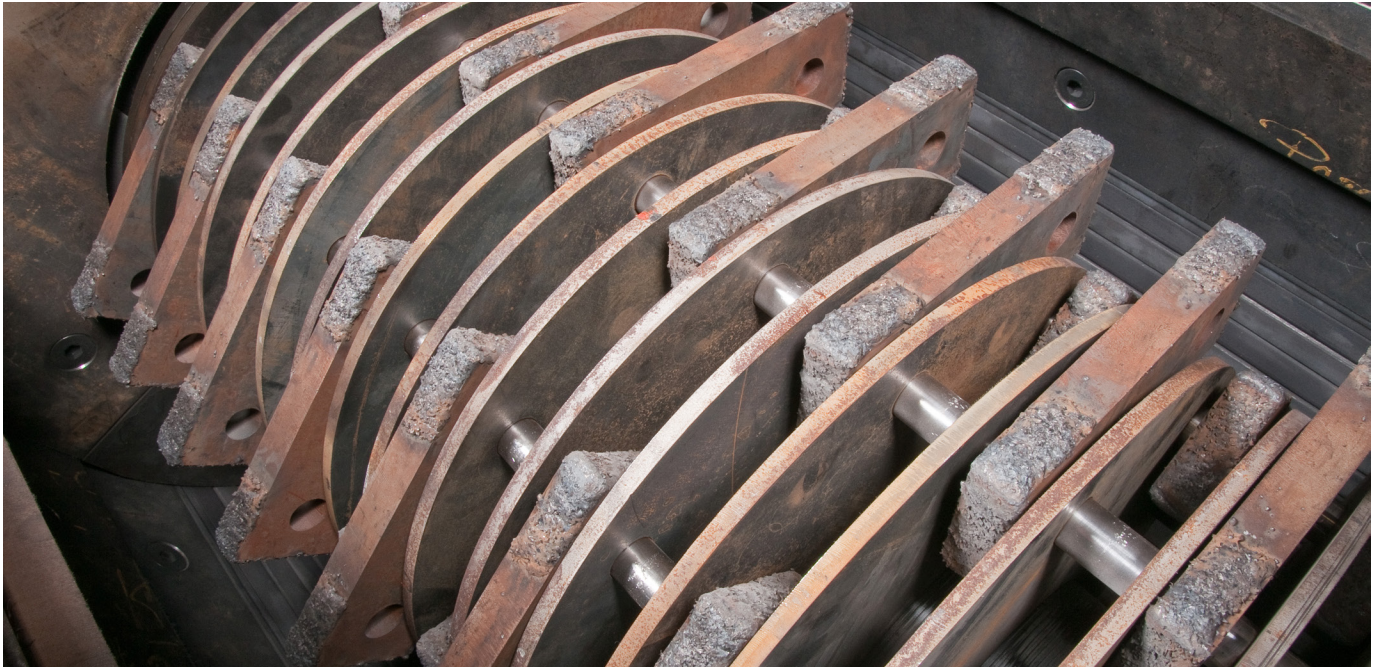
WA Series rotor assembly featuring optional tungsten carbide coated hammers for highly abrasive applications.
