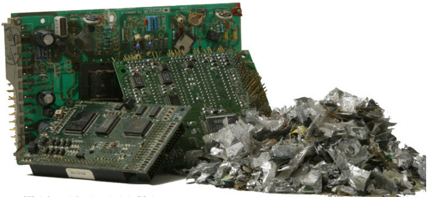
PCBs before and after processing in the E-Cycler
