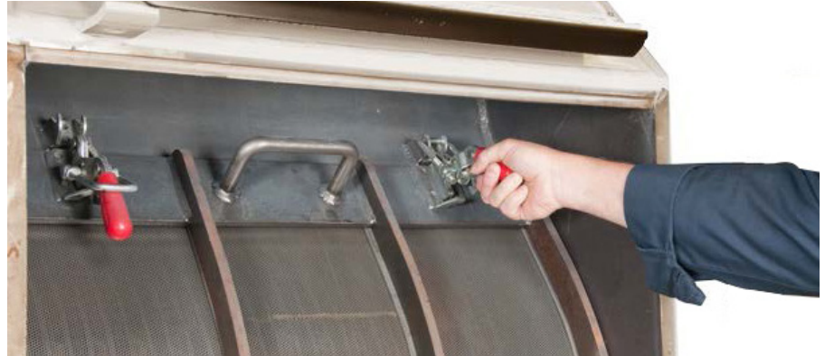
Quick release levers allow for easy screen change, maintenance and rotor inspection.
