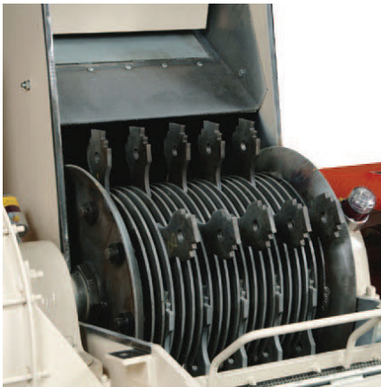
Mill front hinges open for easy screen change, maintenance, and rotor inspection.
