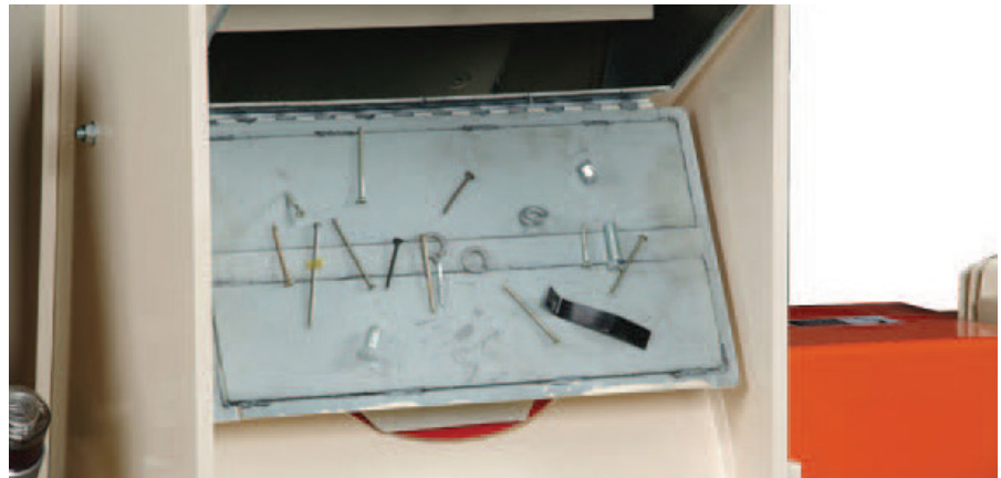
Plate magnet captures all metals before entering the grinding chamber.
