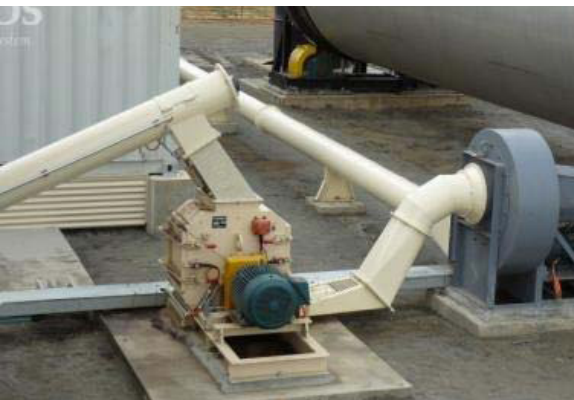
Hammer mill with pneumatic discharge fan and duct to horizontal cyclonic burner.
