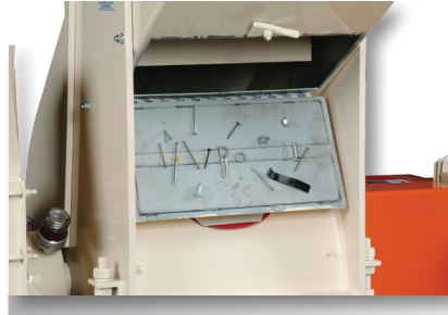
Plate magnet captures all metals before entering the grinding chamber.
