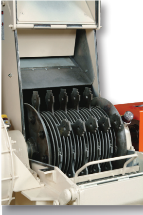
Mill front hinges open for easy screen change, maintenance, and rotor inspection.
