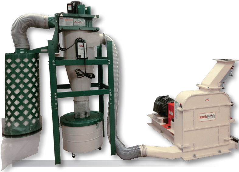
Model 18-7-301 with optional integrated pneumatic discharge system.
