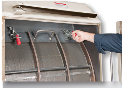
Quick release levers allow for easy screen change, maintenance and rotor inspection.
