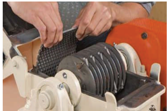
Mill top hinges open for easy screen change and mill maintenance
